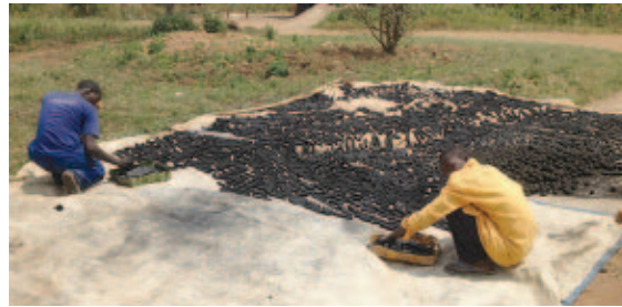
The last step in making this charcoal-like fuel involves drying it in the sun.
